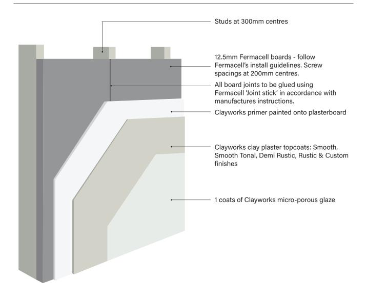
All screws to be filled with joint filler. Follow Fermacell guidelines for internal corners.
