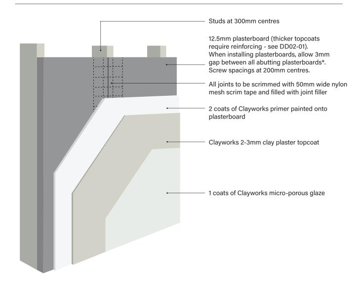
All screws to be filled with joint filler.
