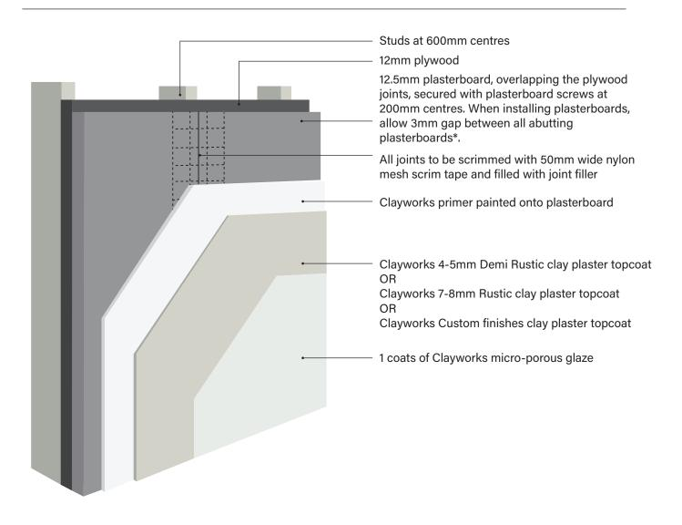
All screws to be filled with joint filler.
