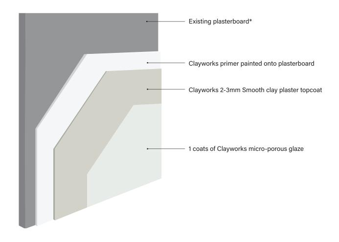
\* If the existing plasterboard has been painted with a plastic-based paint, it will require sanding back before priming.
