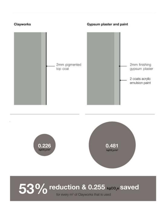
Providing a sense of scale, the chart below shows Clayworks Rustic clay plaster's embodied carbon in comparison with other common building materials. The values here are taken from the Inventory of Carbon and Energy (ICE),<sup>5</sup> an open source database of embodied carbon and energy measurements.
