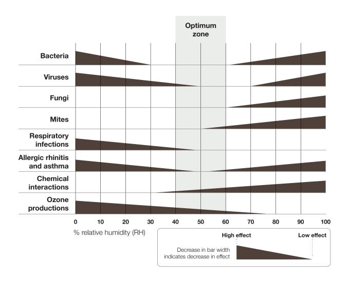
A breathable material, clay plaster is one of the best building materials for maintaining relative humidity within the 'optimum zone' of 40-60%.
