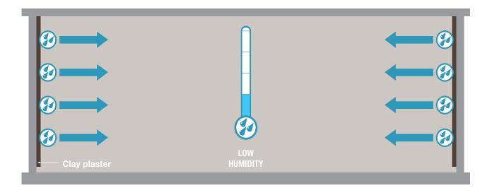
Unfired clay is one of the best materials available when it comes to moisture buffering. Clay has a hygroscopic capacity that is ten times better than gypsum and almost twice as high as lime plaster. Further the speed at which clay is able to absorb and release moisture is much faster than cement, gypsum or lime.<sup>11</sup>
