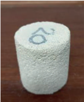
Figure A.1: Test sample as received (BS EN ISO 1182)
