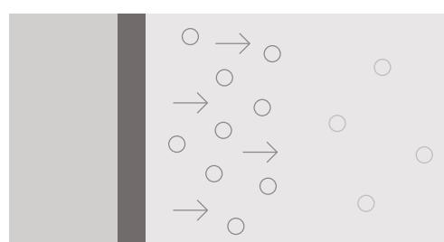
Moisture released by clay surface when relative humidity of a space is low.
