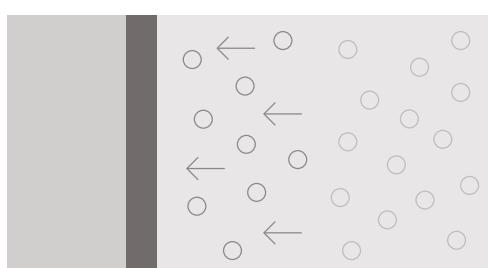
Moisture absorbed and stored by clay surface when relative humidity is high
